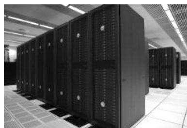
Tungsten Dell PowerEdge 1750 9.82 TFlops, 2500 Xeon 3.06 GHz processors
