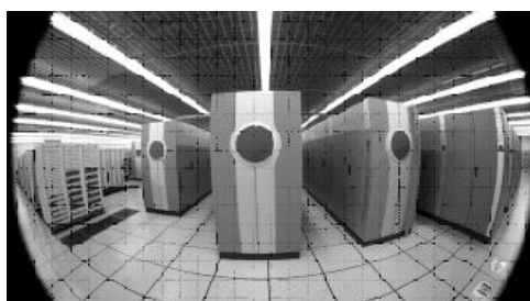
Earth-Simulator 35.86 TFlops, 5120 processors
