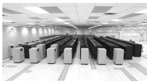
ASCI Q AlphaServer SC45, 1.25 GHz 13.88 TFlops, 8192 processors
