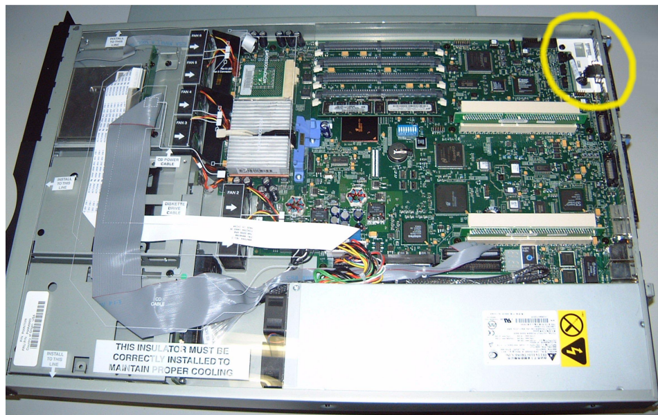
Figure 5-1 x330 as shipped (the serial port connection to be changed is circled)
