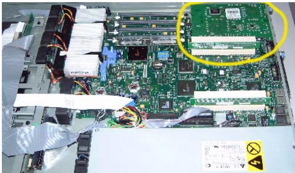
Figure 5-3 x330 with Myrinet card installed into short PCI slot
